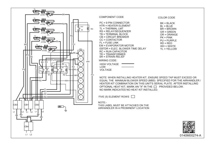
Wiring is subject to change. Always refer to the wiring diagram on the unit for the most up-to-date wiring.
