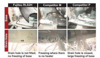
Condition: Indoor temp. of 68°FDB / outdoor temp. of 5°FDB, Heating mode, High airflow volume. Operation for 24 hours.
