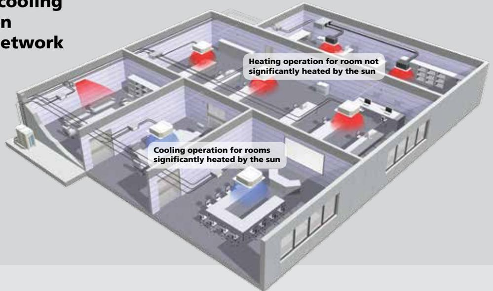
The example below shows two 6-Ton heat pump systems, one operating in full cooling (6 Tons) and one operating in full heating (6 Tons), the power inputs were 5.39kW and 6.08kW respectively, giving a total of 11.47kW. When looking at the same example with a heat recovery system, with 50% of the capacity operating in full cooling (6 Tons) and 50% operating in full heating (6 Tons), the power input for the system can be as low as 4.8kW, this would mean about half reduction in power input.
