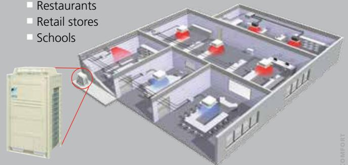
VRVIII is available in heat pump and heat recovery versions where heating and cooling can be made available simultaneously across multiple zones.
