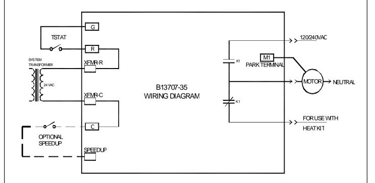
The Electronic Blower Time Delay Relay provides power to the blower motor with a delay of 7 seconds after 24VAC is applied to "G". After 24VAC is removed from "G", the blower motor output is de-energized after a delay of 65 seconds.
