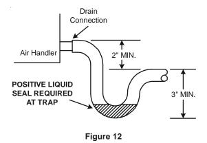
Use of a condensate removal pump is permitted when necessary. This condensate pump should have provisions for shutting off the control voltage should a blocked drain occur. A trap must be installed between the unit and the condensate pump.
