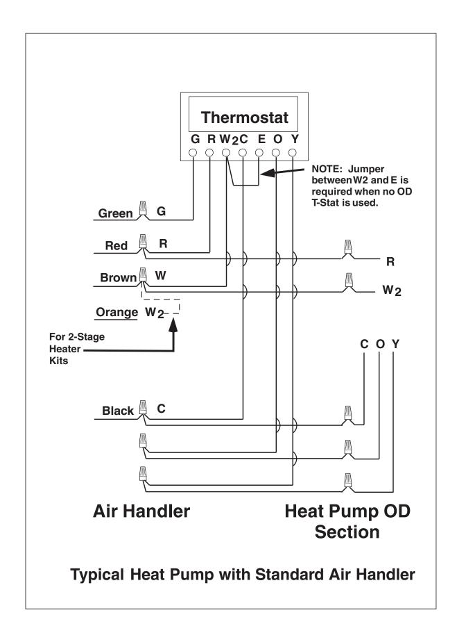
A typical installation with a heat pump thermostat, air handler, and heat pump with an outdoor thermostat.
