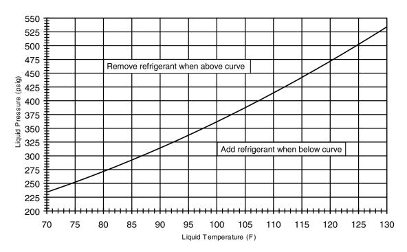
3.5 Ton Heat Pump TXV Cooling Charging Chart
