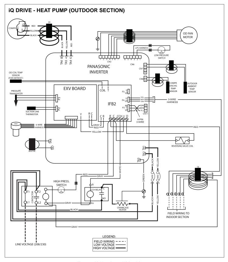
Figure 4. iQ Heat Pump Wiring Diagram
