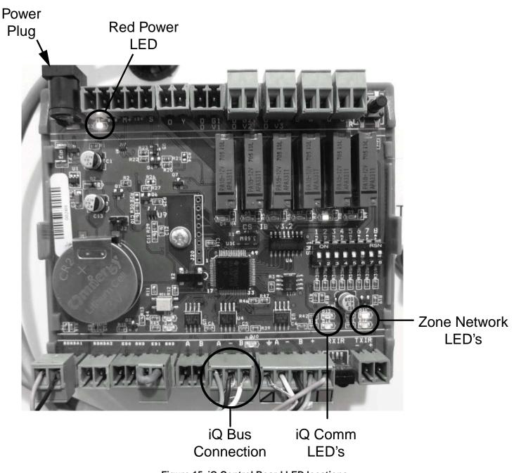
Figure 15. iQ Control Board LED locations
