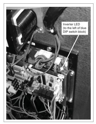
Figure 12. Inverter LED Location (Behind Interface Board, to the left of blue DIP switch block)
