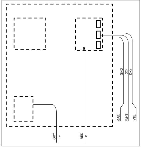
Figure 6. iQ Heat Pump Control Wiring Outdoor Destinations
