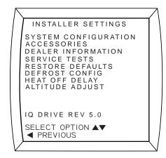
Other than in the splash screen displayed when power is first applied to the controller, this is the only screen which displays the controller software version number. **NOTE:** It is important that any settings or service tests which are appropriate be made at the time of system installation.
