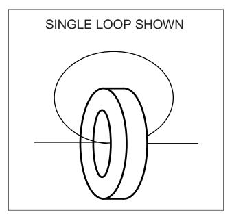
Figure 7. Wire Looping Through a Toroidial Choke
