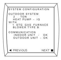
The words under OUTDOOR SYSTEM and WITH describe the system components as automatically detected by the controller. Both entries under COMMUNICATION should show "OK". If "CHECK" appears, it is an indication that either communication wiring is incomplete or incorrect, or the outdoor unit is not powered up. Proceed through subsequent screens by using either the ▶ or ■ key (indicated by "NEXT").
