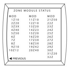
Press the ▶ key to view the ZONE MODULE STATUS screen (shown here). Every module installed in the system should show up on this list with the proper zone identification number after the "Z", followed by a "0". For example, "23Z40" is module 23 in zone 4. The "0" indicates normal functioning. Zone numbers should only appear with module numbers that were intended to be assigned. For master zone modules 1-8, the zone number must match the module number.
