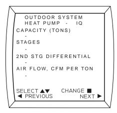
Proceed through the subsequent configuration screens either accepting or changing entries, until the INSTALLER SETTINGS menu is displayed again. This is an indication that configuration has been completed.
