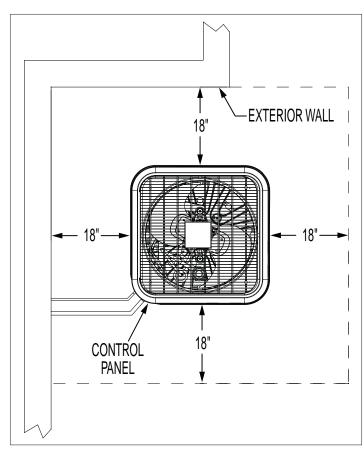
Figure 1. Unit Envelope Dimensions
